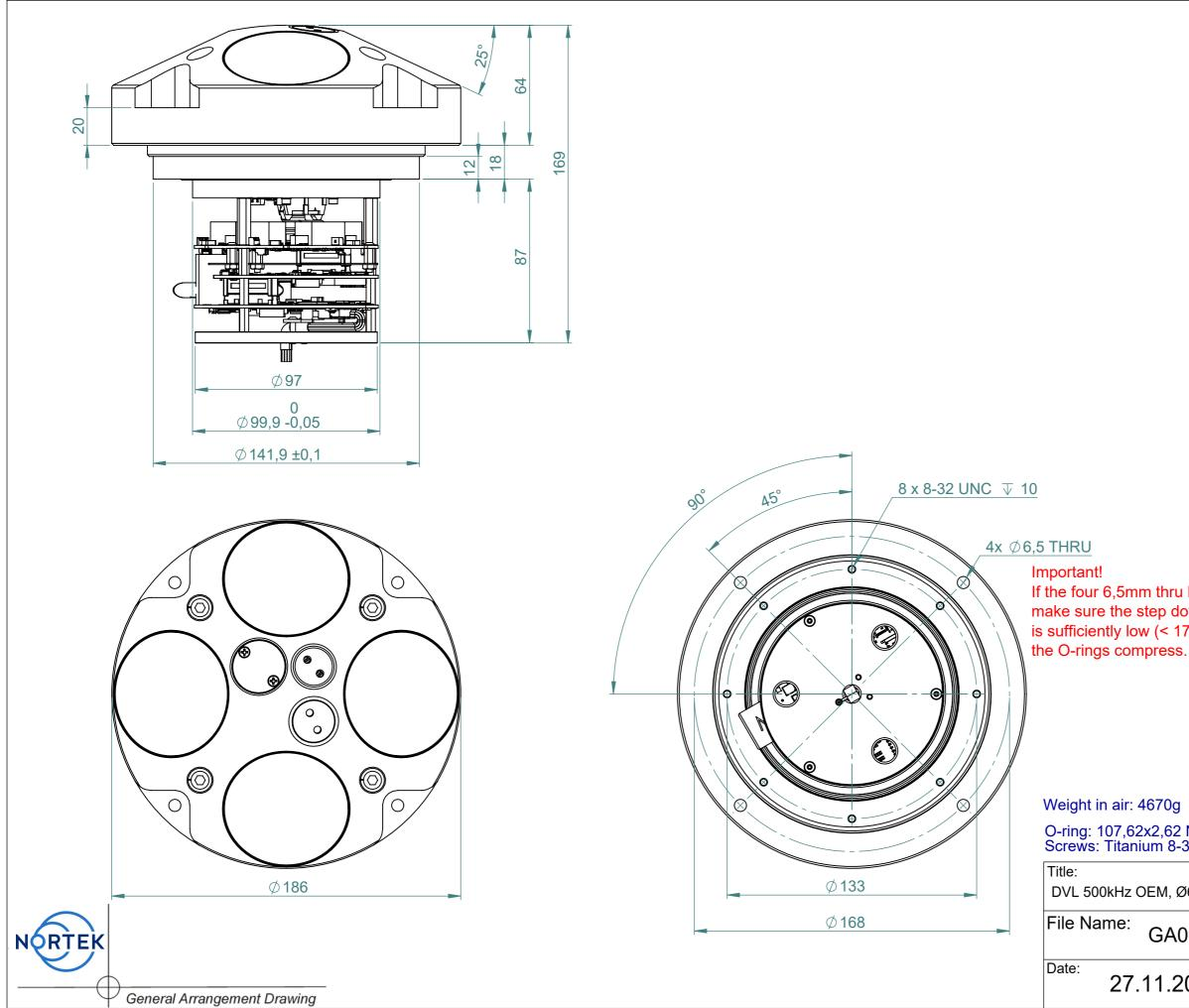
If the four 6,5mm thru holes are used for mounting, make sure the step down to the O-ring sealing surface is sufficiently low (< 17,5mm) in order to make
